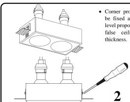
· Corner profiles should be fixed at the height level proportional to the false ceiling panel's
